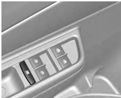
Pressione o interruptor
