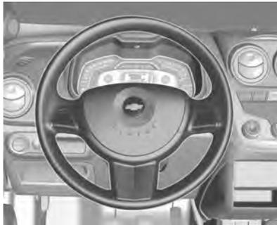
Para veículos equipados com "Airbag", pressione qualquer dos pontos
